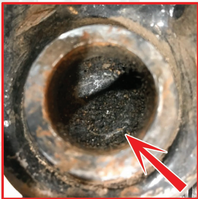
Dry internals showing evidence of ball stud wear (contaminants and old dry grease).
