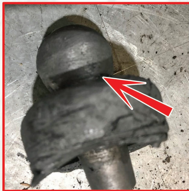
Wear marks on ball stud ball consistent with running without adequate lubrication.
