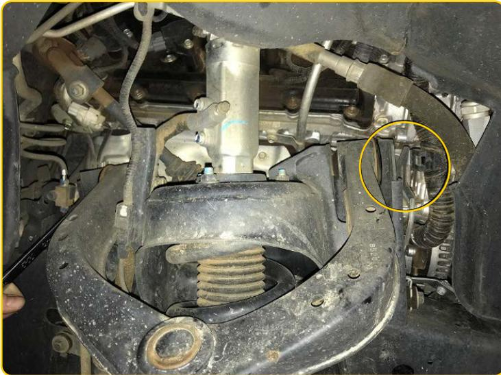
4. There is also a 6mm bolt on the back of the pump that secures the bracket for the wiring loom, remove this also for ease of removing the UCA bolt when you get to it.
