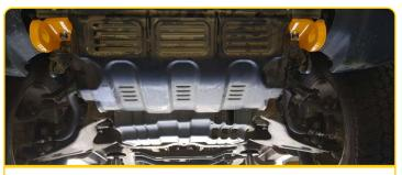
For fitment with factory bash plates, ensure that there is 6mm or more clearance around the recovery point allowing for chassis deflection.
