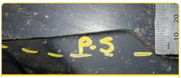
The picture above illustrates trimming required of the passenger side factory bash plate. It is self explanatory once the recovery points are fitted and the bash plate placed in position.
