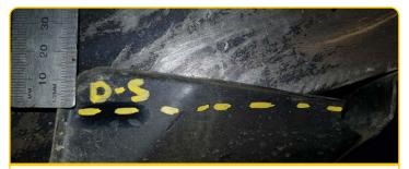
The picture above is of the driver side front bash plate. A similar amount needs to be trimmed. Again placing the bash plate back into position will show how much of this wing needs to be trimmed. Paint cut surface to stop rust forming.
