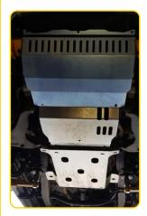
These two pictures are fitment of the RPTRI02 with Roadsafe underbody protection. No modification is necessary.
