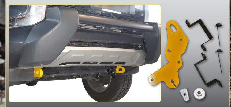
FEA & PHYSICAL DESTRUCTION TESTING COMPLETED WLL 5000KG TESTED IN AUS NATA LAB
