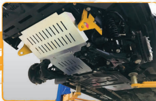
Part Number BP101-3 Ford Ranger PX3 - Third Plate Barcode 9319478660717 Fits at the end of the third (factory) bash plate for Transfer case protection RRP* $149.00
