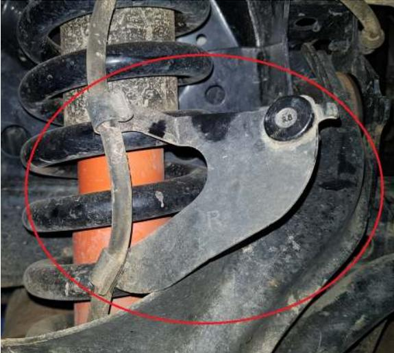
12. Refit brake line clip to the arm using OE nut.
