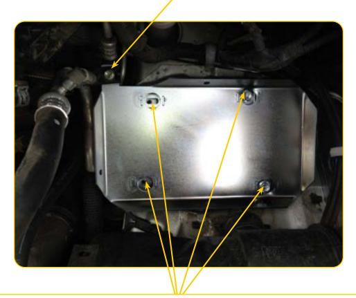
3. Place the 2 x 4mm bolts in the tray in the holes towards the the engine. Then place the 2 x 6mm bolts in the holes towards the guards and tighten all bolts.
