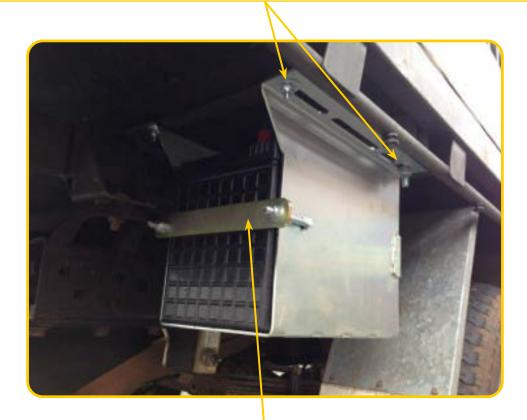
3. Sit battery into box and place battery hold down on. Then tighten until battery is firmly in place.
