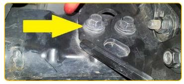
5. This small protruding tab needs to be bent in out of the way for the supplied crush sleeve to fit in. See figure 5.
