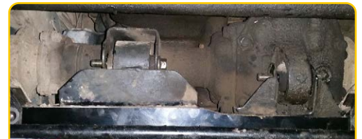
Install supplied dropped cross member with factory diff mounts to vehicle.
