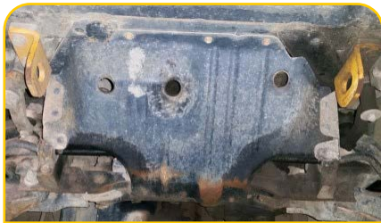
Front factory bash plate to be removed—keep for refitting.
