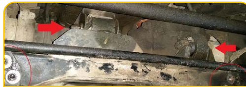
Close up of main X member to be removed & replaced.
