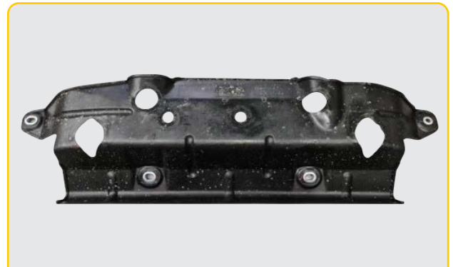
Figure 3 - Notching of plastic undertray
