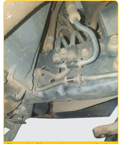
Figure 6 - Clamps that are required to be undone so the lines can be adjusted. SINGLE CAB ANCAP ONLY
