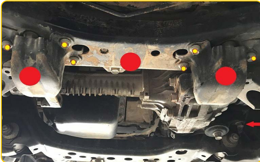
Shows two main spacers installed from rear view
