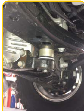
Close up of passenger side main spacer
