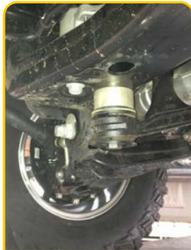
Close up of driver side main spacer
