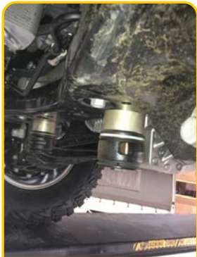
Shows two main spacers installed from rear view
