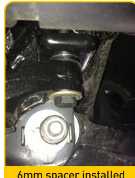
6mm spacer installed into diff mount under passenger side of vehicle
