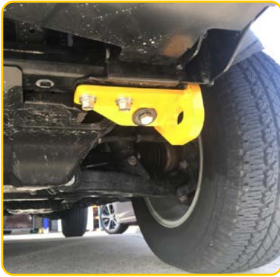
Pic 6. A brake away view of the M12x140 bolt in from the front of the chassis. This is missing the front chassis plate for illustration purposes.
