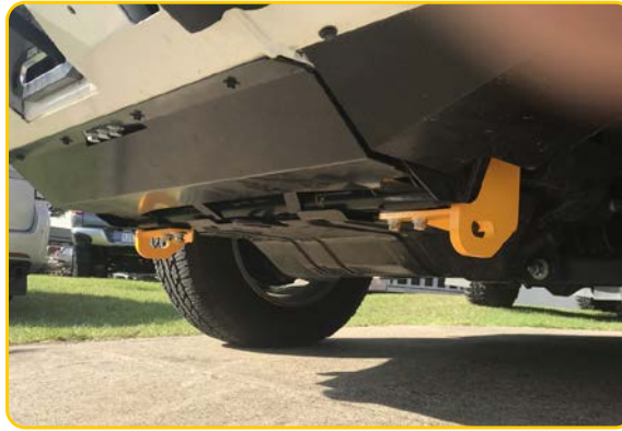
Pic 6. A brake away view of the M12x140 bolt in from the front of the chassis. This is missing the front chassis plate for illustration purposes.
