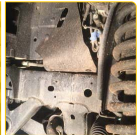
Tuck flaps up in behind chassis rail (out of the way)
