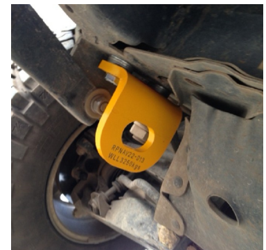
Chassis Gusset for which 12mm Spacer Plates are required
