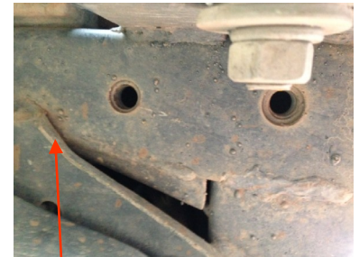
Chassis Gusset for which 12mm Spacer Plates are required
