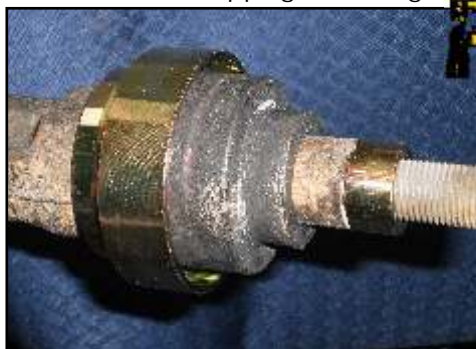
RASWNISV2 fitted to Radius Arm - Increased Cupping of Bushing
