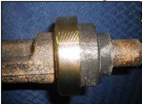
PATRAMBC fitted to Radius Arm - Cups Side Wall of Bushing
